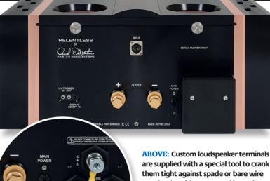
are supplied with a special tool to crank them tight against spade or bare wire terminations [the same tool is used to bolt-down the AC mains cable - see left]. A single balanced XLR input is fitted
