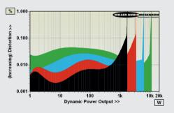
ABOVE: Dynamic power output versus distortion into 80hm (black trace), 40hm (red), 20hm (blue) and 10hm (green) speaker loads. Max. current is 106A (!)
