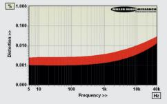
ABOVE: Distortion versus extended frequency (1W/8ohm, black; 100W/8ohm, red)
